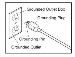
current to reduce the risk of electric shock. This product is equipped with a cord having an equipment-grounding conductor and a grounding plug. Plug the power cord into an appropriate outlet that is properly installed and grounded in accordance with all local codes and ordinances. This product is for use on a nominal 120-volt circuit. Important: The elliptical crosstrainer is not compatible with GFCI-equipped outlets.
